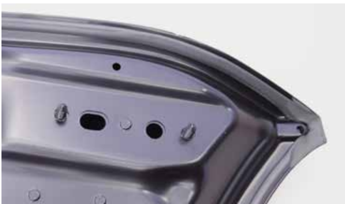
Volkswagen Genuine bonnet with seam sealing.
