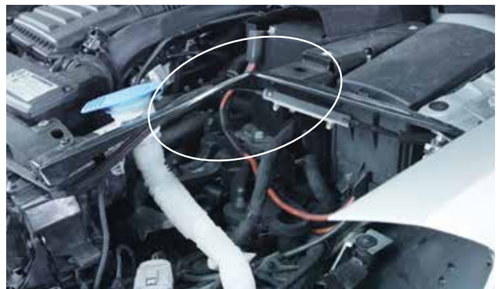
Golf VII with IAM parts. Front mask mounting after the crash: highly bent.
