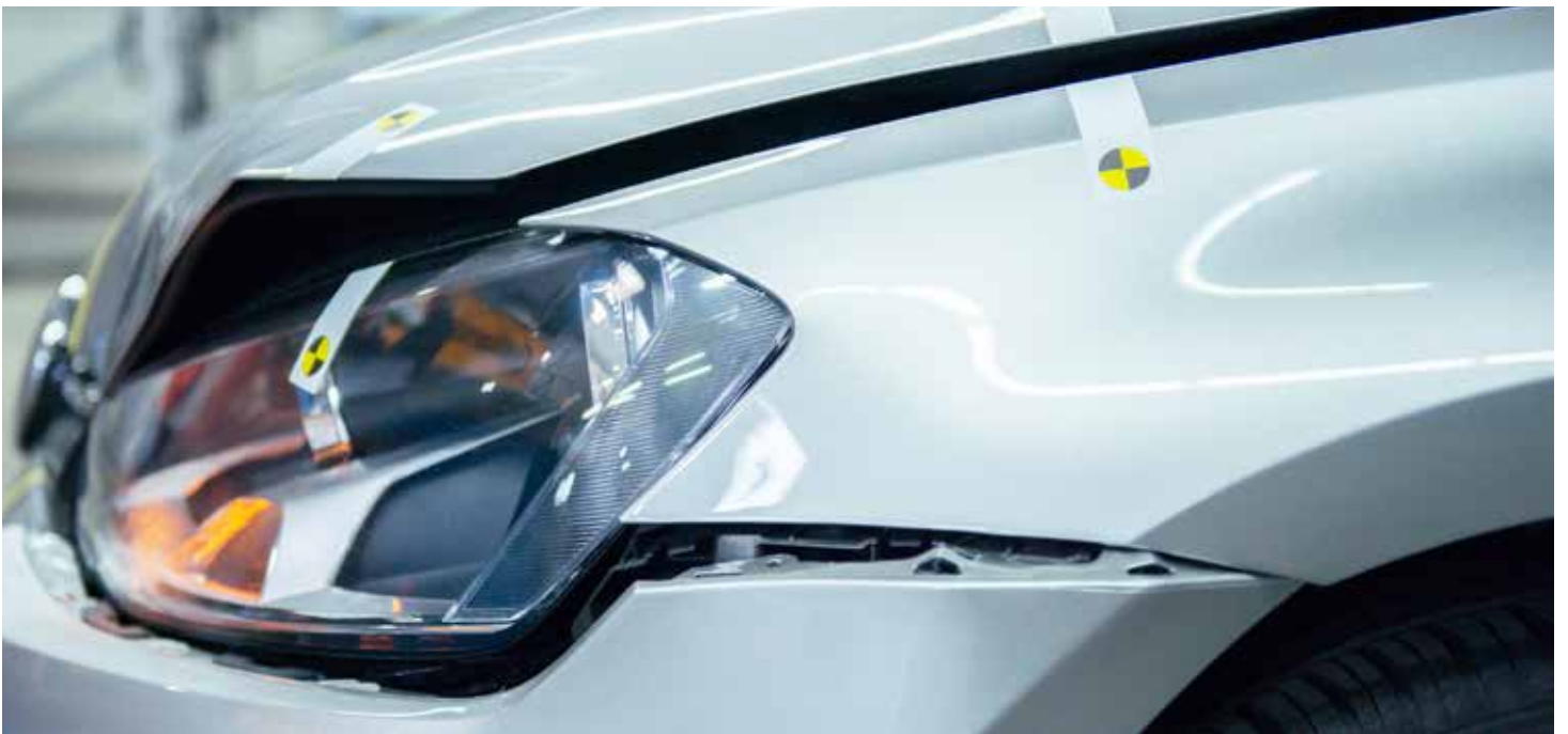
Golf VII with IAM parts. Deformations after the crash.
