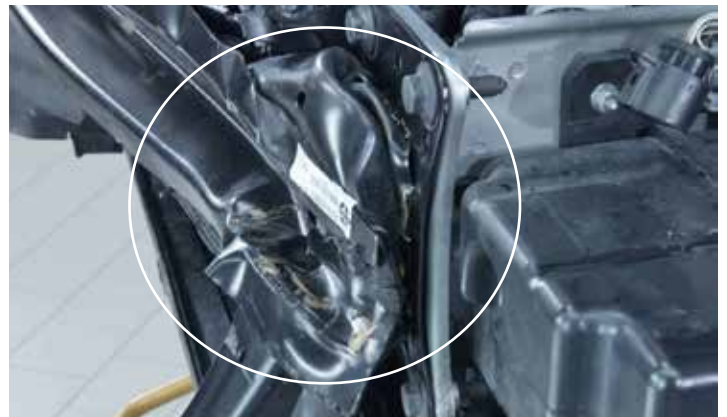
Golf VII with IAM parts. Crashbox dented by 80 mm after the crash.
