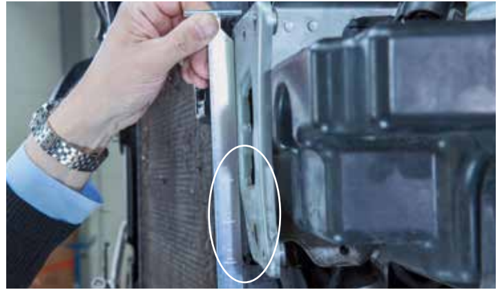
Golf VII with IAM parts. Flange after the crash: adjustment work required.
