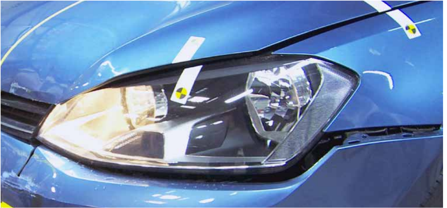
Golf VII with Genuine Parts. Deformations after the crash.
