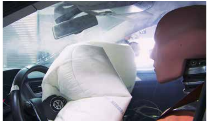
Airbags triggered. Golf VII interior with IAM parts post-crash.
