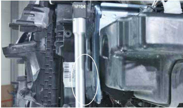
Golf VII with Genuine Parts. Flange after the crash: no adjustment work required.
