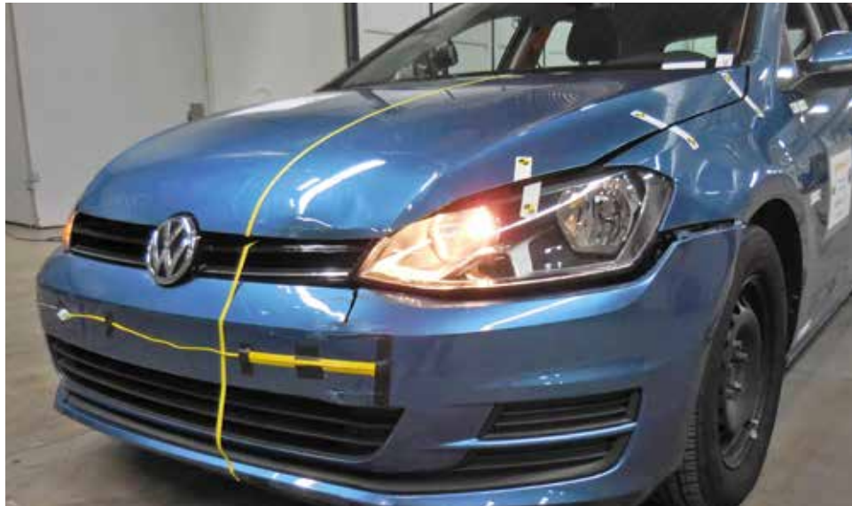
Golf VII equipped with Genuine Parts after the crash test.
