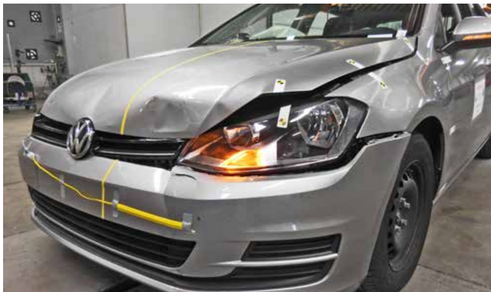
Golf VII equipped with IAM parts after the crash test.
