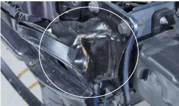
Golf VII with Genuine Parts. Crashbox dented by 37 mm after the crash.
