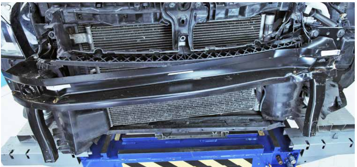
Golf VII with IAM parts. Damages to the front after the crash.
