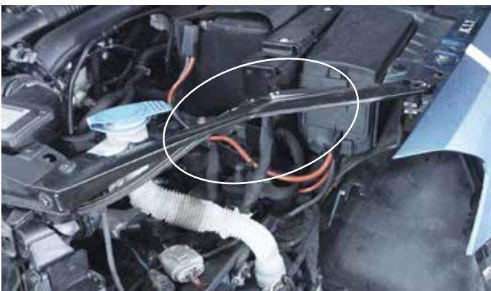
Golf VII with Genuine Parts. Front mask mounting after the crash: lightly bent.
